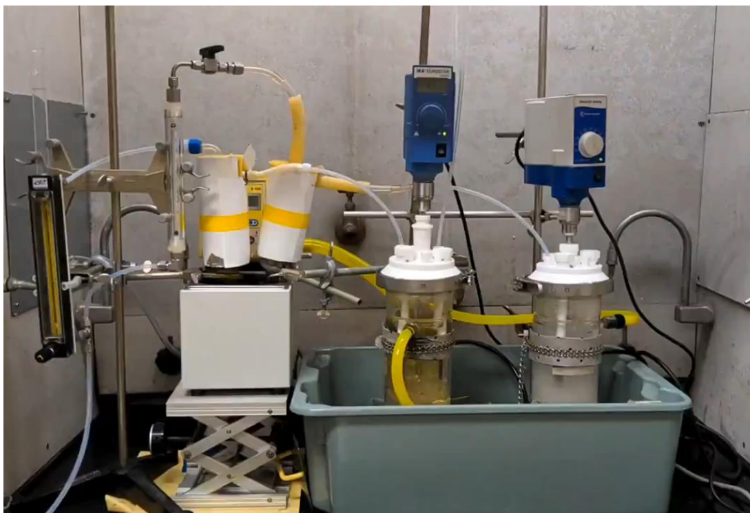
Figure 3-3: Low-gas flow reactor setup
