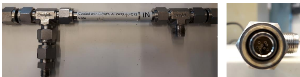
Figure 3: Dense layer membrane integrated in the miniplant
